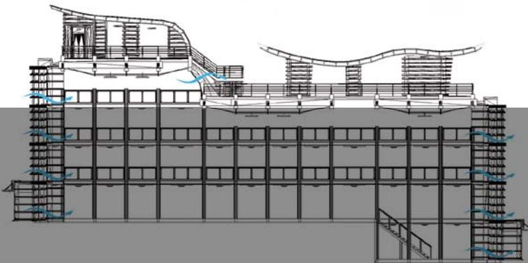
Ventilation diagram - transversal section
